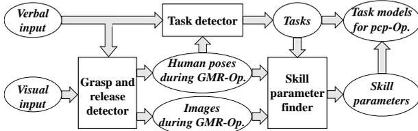
Figure 4. Pipeline used to substantiate the task model.
