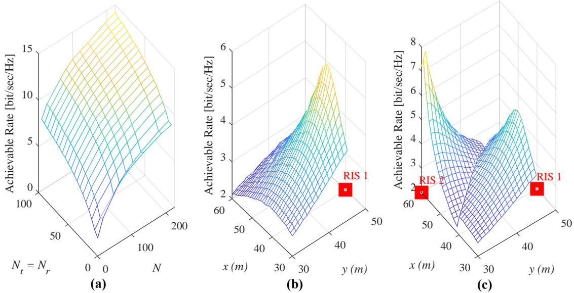
Fig. 5. Achievable rate analysis using SimRIS Channel Simulator: (a) For varying  $N_t/N_r$  and  $N$ , (b) For a single RIS with varying Rx positions, (c) For two RISs with varying Rx positions. Here, the red squares indicate the positions of the RISs on the  $x$  and  $y$ -axes.
