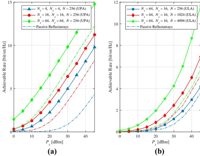
Fig. 4. Achievable rates of RIS-assisted systems (a) in an indoor environment under different  $N_t$  and  $N_r$  with fixed  $N$ , and (b) in an outdoor environment under different  $N$  with fixed  $N_t$  and  $N_r$ .
