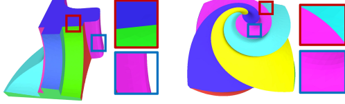
Figure 5. Segmentation on shapes with mixed types of surfaces. Sharp edges (in red frames) are distinguished by our algorithm using two colours, while smooth regions (in blue frames) are marked in the same colour.
