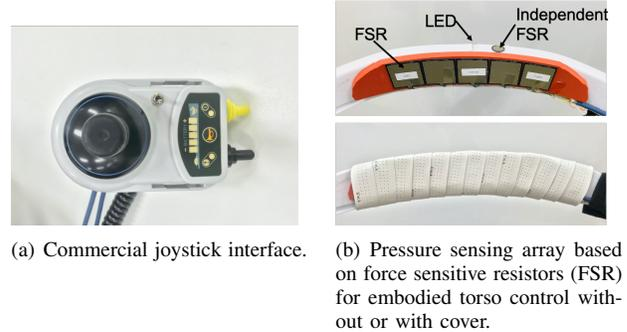
Fig. 4. Pictures of the evaluated motion control interfaces.
