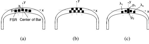
Fig. 3. Distribution examples of pressure sensing matrices, with FSR depicted in black squares. In the current prototype design (a) was selected, however, any configuration would directly work with the proposed algorithms.
