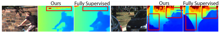
Fig. 7: Failure cases of our method in KITTI, which cannot correct all types of noise. The left side example shows a set of noisy inputs on the wall. The right side example shows dropping of points due to low-reflectance black surfaces
