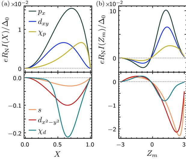
FIG. 5. Thermoelectric effect for the two-dimensional pair potentials listed in Table I. (a) F-I-S junction with  $Z_m = 0$ . (b) F-Fi-S junction with  $X = 0.5$ . In all cases,  $Z_0 = 3$ ,  $T = 0.2T_c$ , and  $\delta T = 0.2T_c$ .
