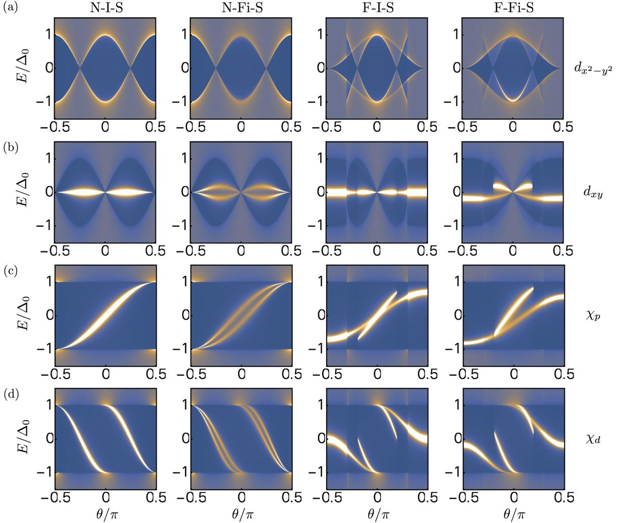
FIG. 4. Spectral differential conductance ( $\sum_{\sigma} P_{\sigma} \sigma_{\sigma} / \sigma_N$ ), where bright colors represent large conductances, for different junctions with the two-dimensional pair potentials (a)  $d_{x^2-y^2}$ -wave, (b)  $d_{xy}$ -wave (c) chiral  $p$ -wave ( $\chi_p$ ) and (d) chiral  $d$ -wave ( $\chi_d$ ). N-I-S and N-Fi-S (F-I-S and F-Fi-S) junctions have  $X = 0$  ( $X = 0.5$ ) and  $Z_m = 0$  and  $Z_m = 2.5$ , respectively. We set  $Z_0 = 5$  in all cases.
