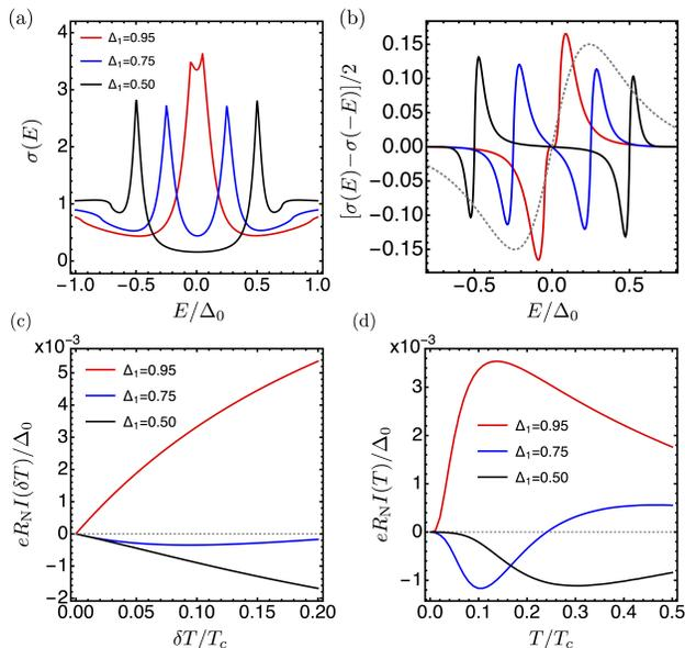
FIG. 3. Conductance (a), its antisymmetric part (b), and the thermoelectric current (c,d) for a two-dimensional junction with  $d_{xy} + is$ -wave pairing. The dotted line in (b) is the difference in Fermi distribution functions for  $T = 0.2T_c$  and  $\delta T = 0.2T_c$ . (c,d) Thermoelectric current as a function of the temperature bias for  $T = 0.2T_c$  (c) and the base temperature with  $\delta T = T/2$  (d). In all cases, we have used  $X = 0.5$ ,  $Z_0 = 3$  and  $Z_m = 0$ .
