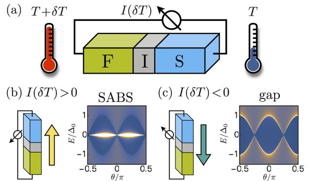
FIG. 1. Thermoelectric effect and direction of the current in a ferromagnet-superconductor hybrid junction. (a) Setup indicating the hot and cold reservoirs. (b,c) Assuming a majority of spin-up particles, a positive thermoelectric current flows into the superconductor (b) in the presence of SABS, while a negative one runs out of it in their absence (c).
