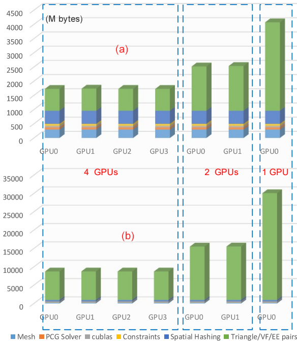
Fig. 13. Memory Overhead vs. Number of GPUs: We highlight the memory overhead (per GPU) of P-Cloth versus the number of GPUs used for simulation for Sphere-1M benchmark: (a) Highlights the average memory utilization by different data structures for a frame without many collisions; (b) Highlights the memory overhead for a frame with a high number of potential self-collisions. This results in a very high number of pairwise tests after spatial hashing. For this benchmark, a single-GPU based algorithm would require about 29 GB and 2-GPU implementation of P-Cloth would need 15 GB on each GPU. On a 4-GPU system, P-Cloth takes up to 8 GB for these challenging close proximity configurations and able to perform the simulation at almost interactive rates. The reduced memory overhead on a multi-GPU system significantly increases the frame rate and performance.
