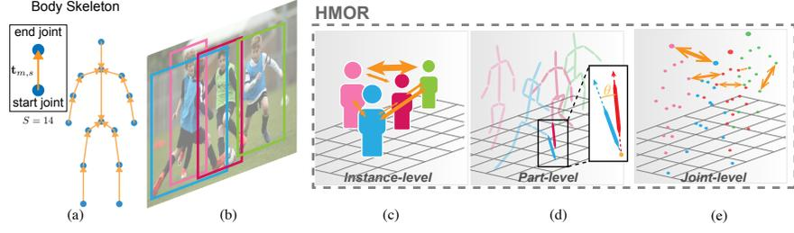
**Fig. 1.** Illustration of the proposed HMOR. (a) Definition of skeletal parts. (b) Monocular input image. (c-e) Hierarchical Multi-person Ordinal Relations. HMOR supervises the ordinal relations among multiple persons
