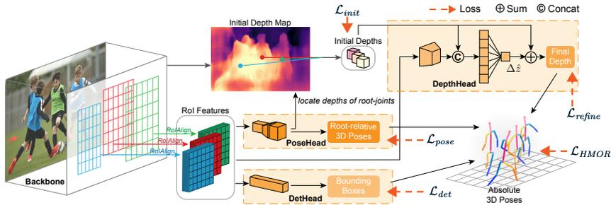
**Fig. 2.** Architecture of the integrated model. The ResNet-50 based backbone network extract RoI features and initial depth map. PoseHead and DetHead perform root-relative 3D pose estimation and human detection, respectively. DepthHead retrieves initial depths from the depth map and predicts refined human depths by correction residual  $\Delta\hat{z}$ . This architecture allows the 2D-3D mixed training strategy
