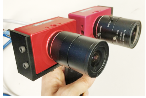
Fig. 10: Custom stereo event-camera rig consisting of two DAVIS346 cameras with a horizontal baseline of 7.5 cm.
