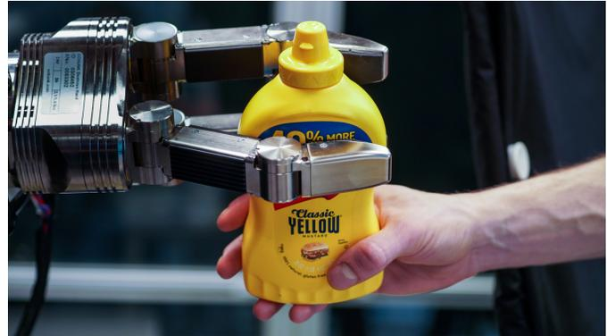
Fig. 1. Example of a direct handover where a robot partner passes a bottle of mustard to a human. As both hands are in contact with the object, this picture shows the physical exchange phase of a handover.
