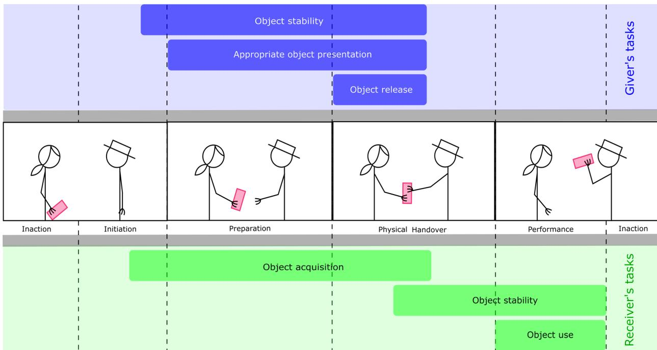
Fig. 2. For each phase of the handover, this figure describes giver's and receiver's tasks.
