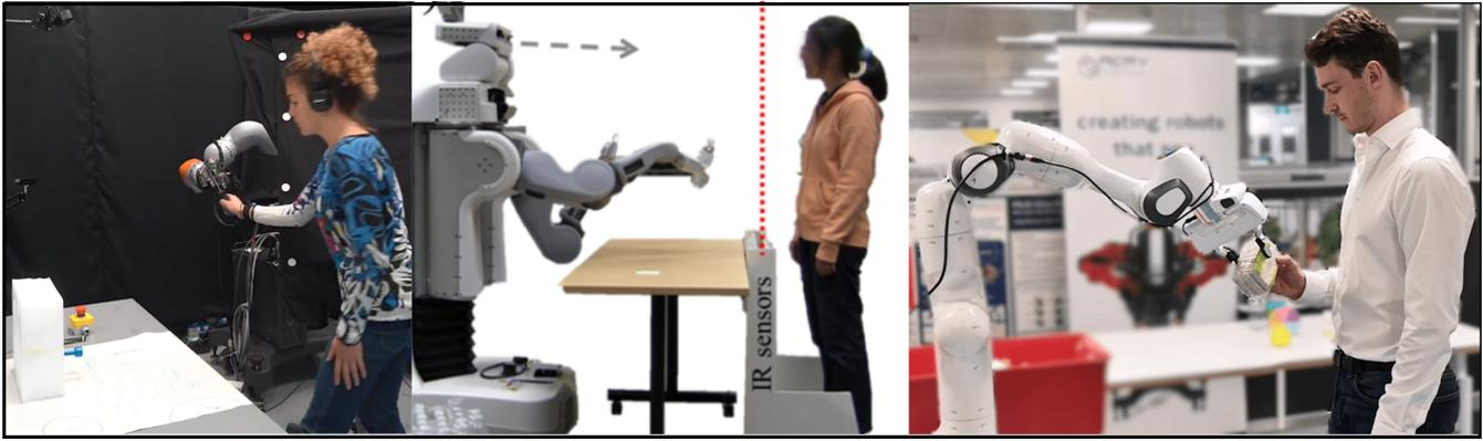
Fig. 4. Examples of real implementations of human-robot handovers. The first two images depict the R2H paradigm, while the rightmost image depicts the H2R paradigm. In all the three instances, a real robot is interacting with the human participant. Images are taken respectively from [93], [48], [118]
