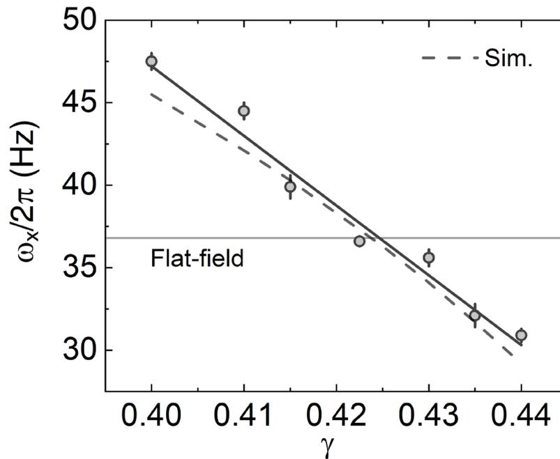
Figure S2: Trend of  $\omega_x/2\pi$  versus  $\gamma$ . Gray points are the experimental measurements at  $E_{DC} = 5$  kV/cm, solid gray line is a linear fit to guide the eye, and dashed line is the prediction from the finite-element model.
