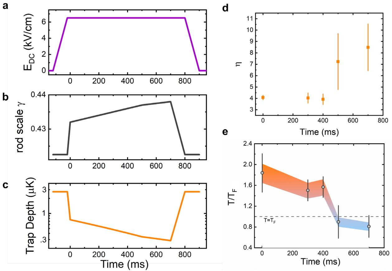
**Figure S3:** **a**, Ramp in  $E_{DC}$ . **b**, Ramp in  $\gamma$ . **c**, Trap depth vs time from the finite-element model of electro-optical potential. **d**, Evolution of  $\eta$ , from taking the ratio of the trap depth and temperature at each time-point. **e**, Evolution of  $T/T_F$  during the ramp.
