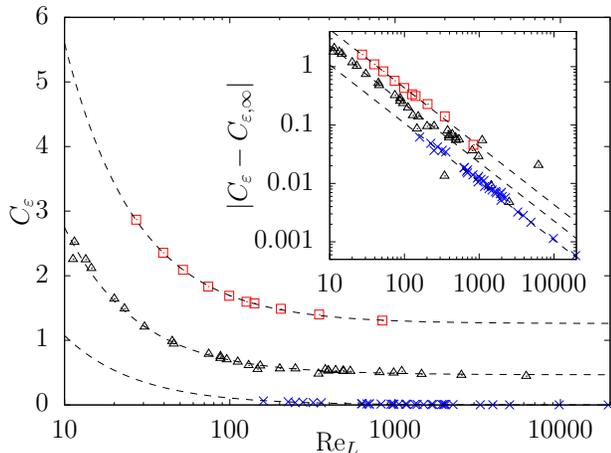
FIG. 5: Main panel:  $C_\varepsilon$  against  $Re_L$ . Dashed line fit for model Equation (6) for two ( $\times$ ), three ( $\Delta$ ) and four ( $\square$ ) dimensions. Inset:  $|C_\varepsilon - C_{\varepsilon,\infty}|$  against  $Re_L$ , dashed line corresponds to power law behavior.
