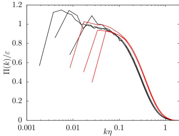
FIG. 2: (Color online) Normalized energy flux,  $\Pi(k)$  against  $k\eta$  at  $\text{Re}_L = 6207, 2517$  and  $979$  for 3D (black) and  $\text{Re}_L = 838, 347$  and  $203$  for 4D (red).
