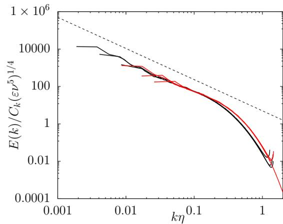
FIG. 1: (Color online) Normalized energy spectrum,  $E(k)$ , against  $k\eta$  at  $Re_L = 6207, 2517$  and  $979$  for 3D (black) and  $Re_L = 838, 347$  and  $203$  for 4D (red). Kolmogorov  $k^{-5/3}$  predicted inertial range scaling (long-dashed black).
