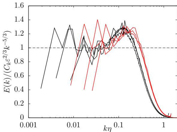
FIG. 3: (Color online) Log-linear plot of compensated energy spectrum,  $E(k)$ , against  $k\eta$  at  $\text{Re}_L = 6207, 2517$  and  $979$  for 3D (black) and  $\text{Re}_L = 838, 347$  and  $203$  for 4D (red).
