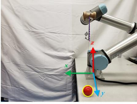
Fig. 1. Manipulator with Kendama along with coordinate frame.
