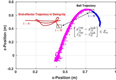
Fig. 2. Start of catch phase (i.e.,  $i = N$ ) for 100 trajectories. Red line indicates the trajectory of the cup/end-effector during swing-up. Blue dots indicate ball positions during swing-up and pink dots indicate a position after catch phase is started. Closed-loop control begins when the relative position is in  $\mathcal{E}_{\text{tr}}$ .
