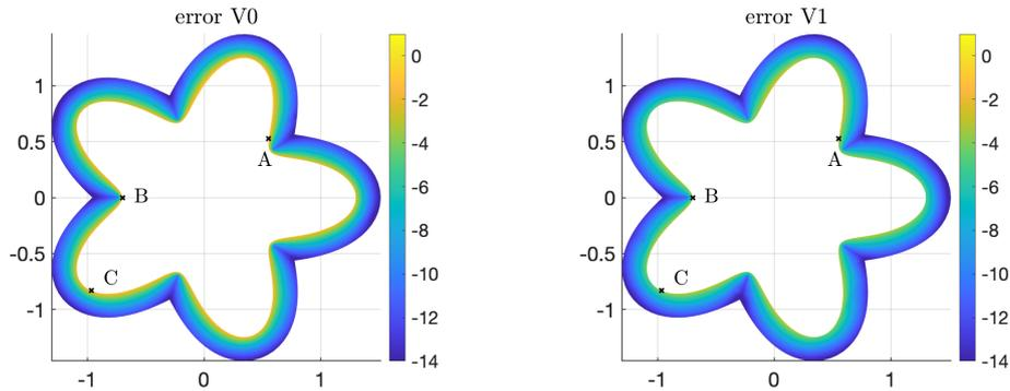
FIGURE 6 – **Helmholtz 2D**. Plots of  $\log_{10}$  of the error for the evaluation of the solution of (18) out of the star domain defined by the boundary  $y(t) = (1 + 0.3 \cos 5t) * (\cos t, \sin t)$ ,  $t \in [0, 2\pi]$ , for the Dirichlet data,  $f(x^*) = \frac{i}{4} H_0^{(1)}(15|x^* - x_0|)$  with  $x_0 = (0.2, 0.8)$ , for representations V0, V1, computed using PTR with  $N = 256$ .
