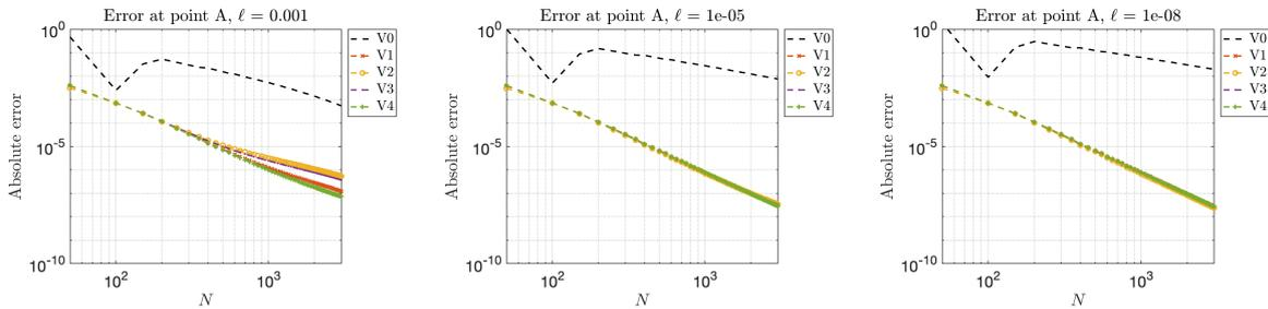
FIGURE 3 – **Laplace 2D single-layer**. Log-log plots of the errors with respect to  $N$  made in computing the solution at some distance  $\ell$  along the normal from the point A plotted as black  $\times$ 's in Figure 1.
