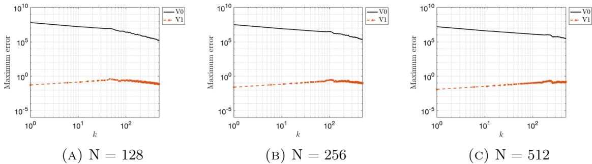
FIGURE 11 – **Helmholtz 2D**. Log-Log of the maximum error in computing the solution of Problem (18) as described in Section 4.2.1, with respect to the wavenumber  $k$ , for various number of quadrature points  $N$ .
