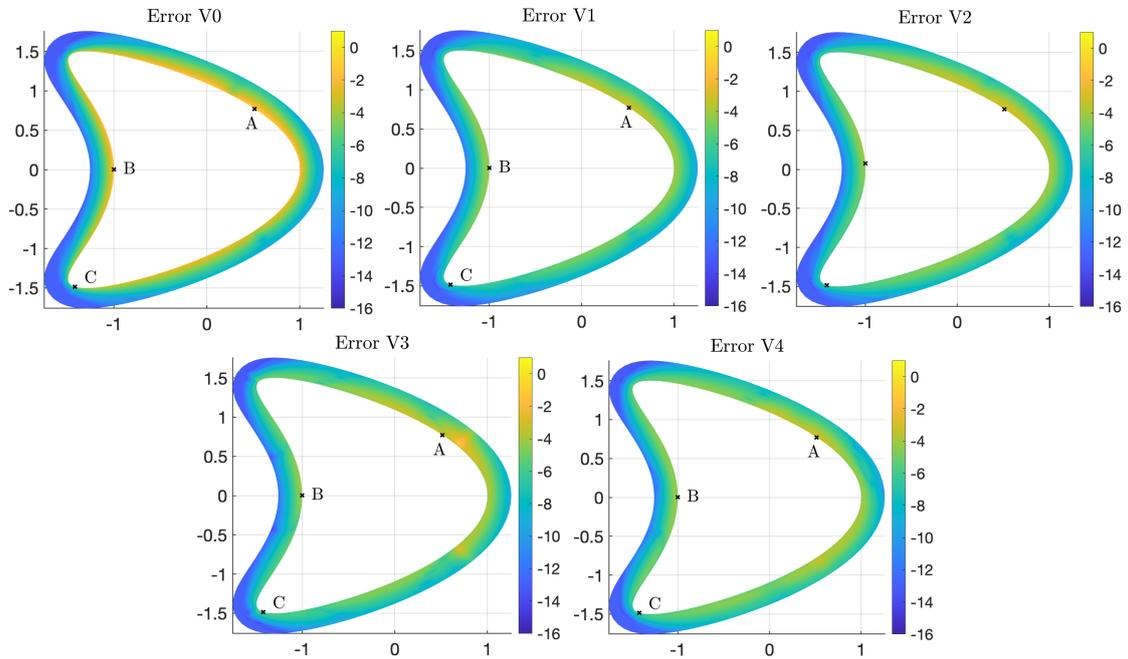
FIGURE 1 – **Laplace 2D single-layer**. Plots of  $\log_{10}$  of the error for the evaluation of the solution of (2) out of the kite domain defined by the boundary  $y(t) = (\cos t + 0.65 \cos(2t) - 0.65, 1.5 \sin t)$ ,  $t \in [0, 2\pi]$ , for the Neumann data,  $g = \partial_n u_{\text{exact}}$  with  $x_0 = (0.1, 0.4)$ , for representations V0, V1, V2, V3, V4 computed using PTR with  $N = 128$ . Computations are made on a body-fitted grid with  $N \times 200$  grid points.
