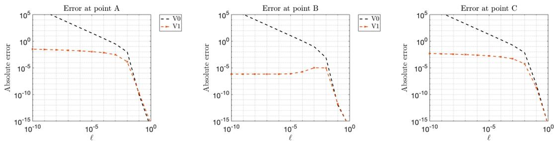
FIGURE 7 – **Helmholtz 2D**. Log-log plots of the errors made in computing the solution along the normal of the three points A, B, C, plotted as black  $\times$ 's in Figure 6.
