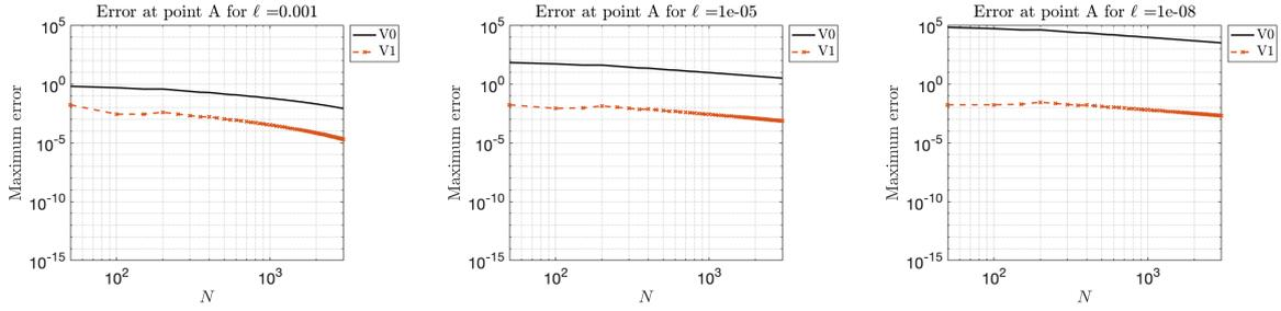
FIGURE 8 – **Helmholtz 2D**. Log-log plots of the errors with respect to  $N$  made in computing the solution at some distance  $\ell$  along the normal from the point A plotted as black  $\times$ 's in Figure 6.
