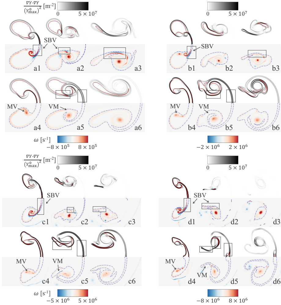
FIGURE 30. Scalar dissipation rate with red isoline of Y_{\text{He}} = 95\% Y_{\text{max}}^0 (top) and vorticity with blue isoline of Y_{\text{He}} = 5\% Y_{\text{max}}^0 (bottom) for (a) Ma = 1.22 ; (b) Ma = 1.8 ; (c) Ma = 3 ; (d) Ma = 4 . For each Mach number, 1 – 3 indicate VD SBI and 4 – 6 indicate PS SBI at three same moments marked as three blue circles in figure 6. Specifically, t = 58 \mu\text{s} , 96 \mu\text{s} , 176 \mu\text{s} for Ma = 1.22 ; t = 19.2 \mu\text{s} , 43.2 \mu\text{s} , 59.2 \mu\text{s} for Ma = 1.8 ; t = 11 \mu\text{s} , 19.8 \mu\text{s} , 26.4 \mu\text{s} for Ma = 3 ; t = 8 \mu\text{s} , 20 \mu\text{s} , 27.2 \mu\text{s} for Ma = 4 .
