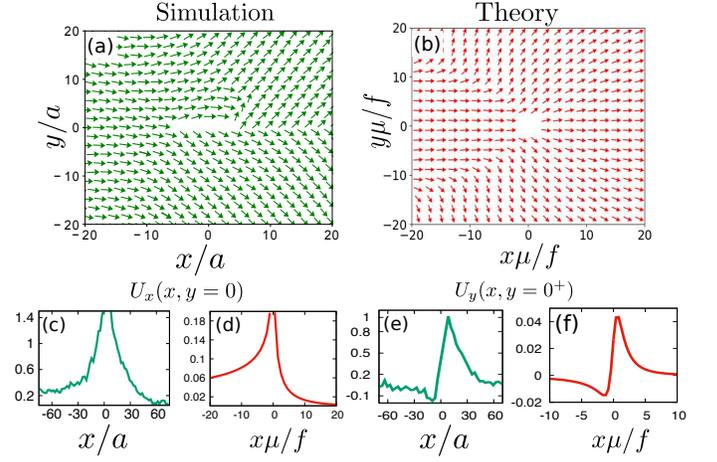
FIG. 1. Normalized displacement field: (a) around a moving rod in the crystalline bead medium from the simulation, and (b) around a force monopole moving along the  $x$  direction calculated from the theory. (c) & (d)  $x$  dependence of  $U_x$  at  $y = 0$  in simulation and theory: both cases see the rapid decay of  $U_x(x, y = 0)$  for  $x > 0$  as compared to  $x < 0$ . (e) & (f)  $x$  dependence of  $U_y$  at  $x = 4a$  in simulation and at  $y\mu/f = 1$  in theory.
