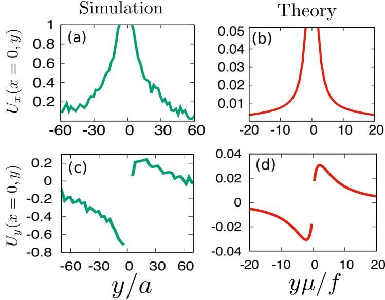
Supplementary Figure 1. Displacement field decay profile: (a) & (b)  $y$  dependence of  $U_x$  at  $x = 0$  in simulation and theory: symmetrical decay of  $U_x(x = 0, y)$ . (c) & (d)  $y$  dependence of  $U_y$  at  $x = 0$  in simulation and in theory.
