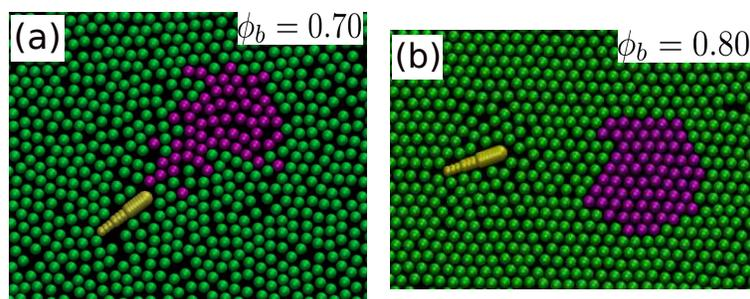
Supplementary Figure 4. (a) Dragging of surrounding beads (marked purple) by the rod due to their fluid-like state of organization at  $\phi_b = 0.70$ . (b) At  $\phi_b = 0.80$ , the beads around the rods remain almost unperturbed because of the crystalline nature of the bead medium.
