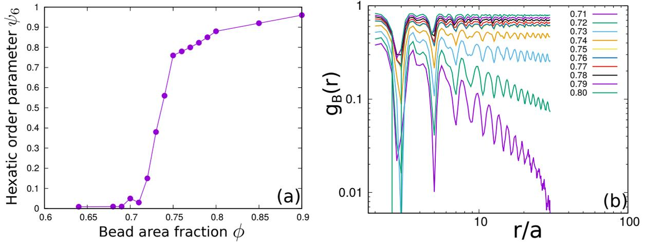
Supplementary Figure 2. (a)  $\psi_6$  order parameter as a function of bead area fraction  $\phi_b$ . (b) Bond orientational correlation function vs distance  $r$  scaled by bead radius  $a$  at different values of  $\phi_b$ .
