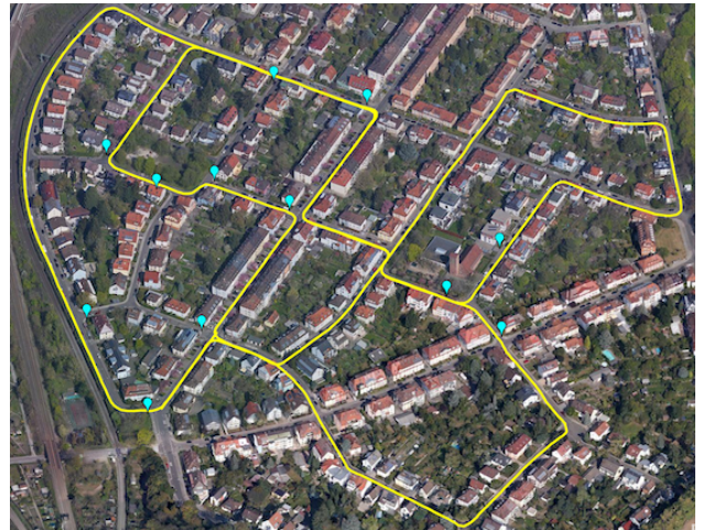
Fig. 1. 3D traffic sign triangulation in Germany without prior knowledge of camera parameters. The estimated signs are shown in cyan. The computed path of the vehicle used for triangulation is depicted in yellow.
