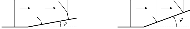
Figure 2: Schematic of Mach (left) and regular (right) reflection of a soliton impinging upon a compressive corner.
