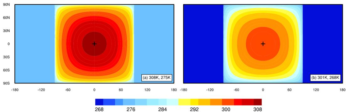
**Fig. 6.** Surface air temperatures specified in the simulations of planets in the middle range of the habitable zone. (a): Maximum surface temperature is 308 K and the night-side surface temperature is uniform with a value of 275 K. (b): Same as (a) but the temperature is 7 K lower throughout.
