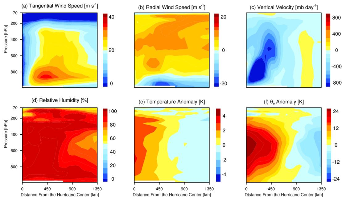
**Fig. 2.** Azimuthal-mean height-radius cross-section of a typical, mature hurricane on the day side of a tidally locked aqua-planet in the control experiment. (a) tangential wind speed ( $v_\theta$ ), (b) radial wind speed ( $v_r$ ), (c) vertical velocity ( $\omega$ ), (d) relative humidity, (e) temperature anomaly from the environmental value ( $\Delta T$ ), and (f) equivalent potential temperature anomaly ( $\Delta\theta_e$ ).
