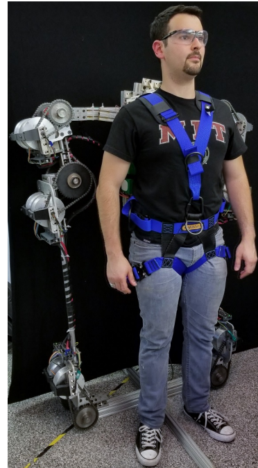
Fig. 1: The Prototype Extra Robotic Legs (XRL) System being worn by an operator.
