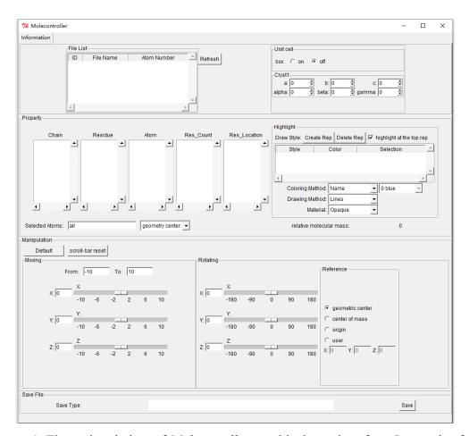
**Figure 1.** The main window of *Molcontroller* graphical user interface. It contains four function boxes: *Information*, *Property*, *Manipulation* and *Save File*.
