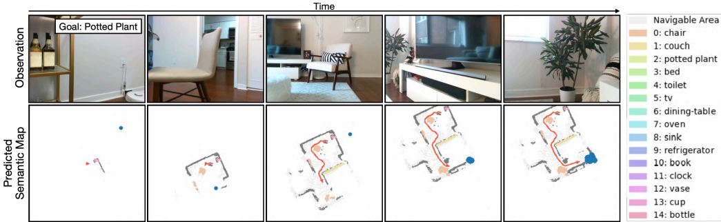
Figure 6: Real-world Transfer. Figure showing an example trajectory of the SemExp model transferred to the real-world for the object goal ‘potted plant’. Sample images seen by the robot are shown on the top and the predicted semantic map is shown below. The long-term goal selected by the Goal-driven Policy is shown in blue.
