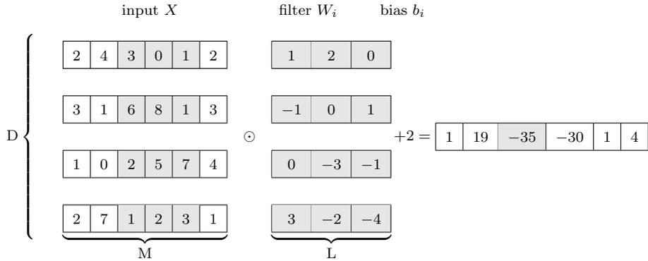
Figure 2: Illustration of a 1-dimensional convolution on an input width  $M=6$ , height  $H=1$ , and depth  $D=4$ . This is equivalent to a 2-dimensional convolution on an input of width 6, height 4, and depth 1. The filter “slides” from the left to the right.
