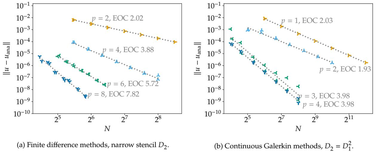
Figure 6: Convergence results of the spatial semidiscretizations (4.39) with  $D_4 = D_2^2$  for the manufactured solution (4.8) of the HH equation. All of these semidiscretizations conserve the linear and quadratic invariants (4.38) of the HH equation (4.36).
