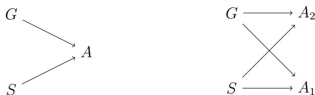
Figure 9. Left , schematic of the policy in Eq. 13, where the behavioral goal G and the perceptual state S jointly determine a single atomic action A . Right , a policy where the behavioral G and the perceptual state S determine two actions A_1 and A_2 to be performed by different actuators.
