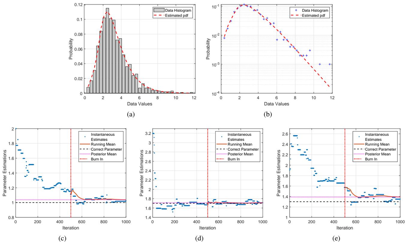
Fig. 3. Modeling and parameter estimation results for synthetically generated data for the GG-Rician model of (1, 1.7, 1.3). (a) pdf Fitting. (b) Log-pdf fitting. Instantaneous estimates are presented for (c) The shape parameter  $\alpha$ , (d) The location parameter  $\delta$ , and (e) The scale parameter  $\gamma$ .
