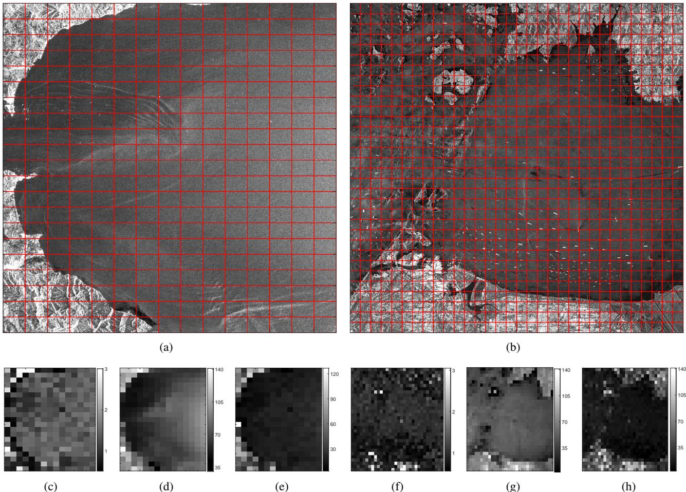
Fig. 10. Estimated model parameters for two large SAR scenes for  $250 \times 250$  image patches in red rectangles. (a) Original Image-1 ( $5250 \times 3750$ ). (b) Original Image-2 ( $8000 \times 8000$ ). (c) and (f) The shape parameter  $\alpha$ . (d) and (g) The location parameter  $\delta$ . (e) and (h) The scale parameter  $\gamma$ .
