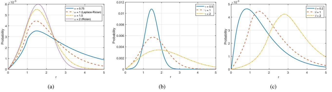
Fig. 2. The proposed GG-Rician distribution pdfs for different model parameters of (a) the shape parameter  $\alpha$  ( $\gamma = 1$  and  $\delta = 1$ ), (b) the scale parameter  $\gamma$  ( $\alpha = 1.7$  and  $\delta = 1$ ), and (c) the location parameter  $\delta$  ( $\alpha = 1$  and  $\gamma = 1$ ).
