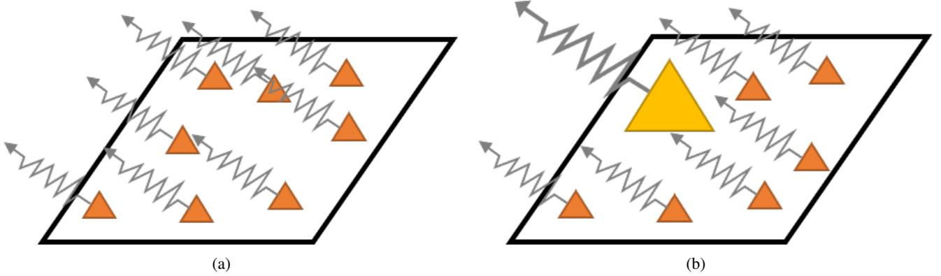
Fig. 1. Surface scattering examples for radar signals. (a) Distributed scattering from multiple scatterers, (b) A scene includes a single dominating scatterer as well as multiple distributed ones.
