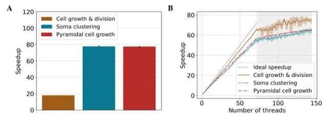
**Fig. 6. BioDynaMo performance analysis.** (A) Speedup of BioDynaMo compared to Cortex3D. (B) Strong scaling behavior of BioDynaMo on a server with 72 physical cores, two threads per core, and four NUMA domains. The grey area highlights hyper-threads.
