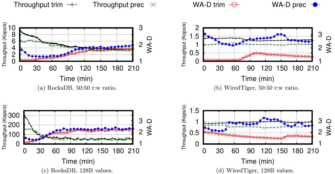
Figure 11: Performance of RocksDB (left) and WiredTiger (right) over time, with a preconditioned and trimmed device. The top row refers to a workload with small (128 bytes) values. The bottom row refers to a workload with a 50:50 read:write ratio. The pitfall we describe apply to a broad set of workloads as long as they have a sustained write component (here we represent pitfalls #1, #2 and #3).
