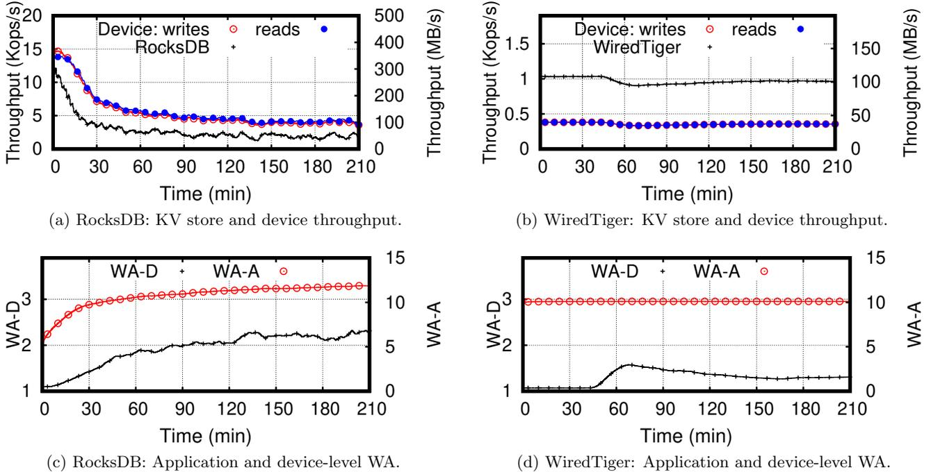
Figure 2: Difference between steady state and bursty performance (on a trimmed SSD) in RocksDB (left) and WiredTiger (right). Steady-state performance differs from the initial one (top) because of the change in write amplification (bottom).
