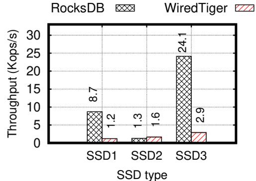
Figure 9: Impact of the SSD type on the throughput of RocksDB and WiredTiger. The type of SSD significantly affects the absolute performance achieved by the two systems, and can even determine which of them achieves the higher throughput.
