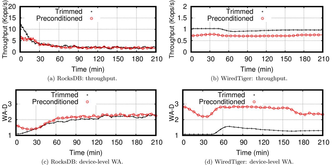
Figure 3: Impact of the initial state of the SSD on performance. Performance achieved over time by RocksDB (left) and WiredTiger (right) depending on the initial conditions of the SSD (trimmed versus preconditioned). The initial conditions of the drive affect throughput (top), potentially even at steady-state, because they affect SSD garbage collection dynamics and the corresponding WA-D (bottom).
