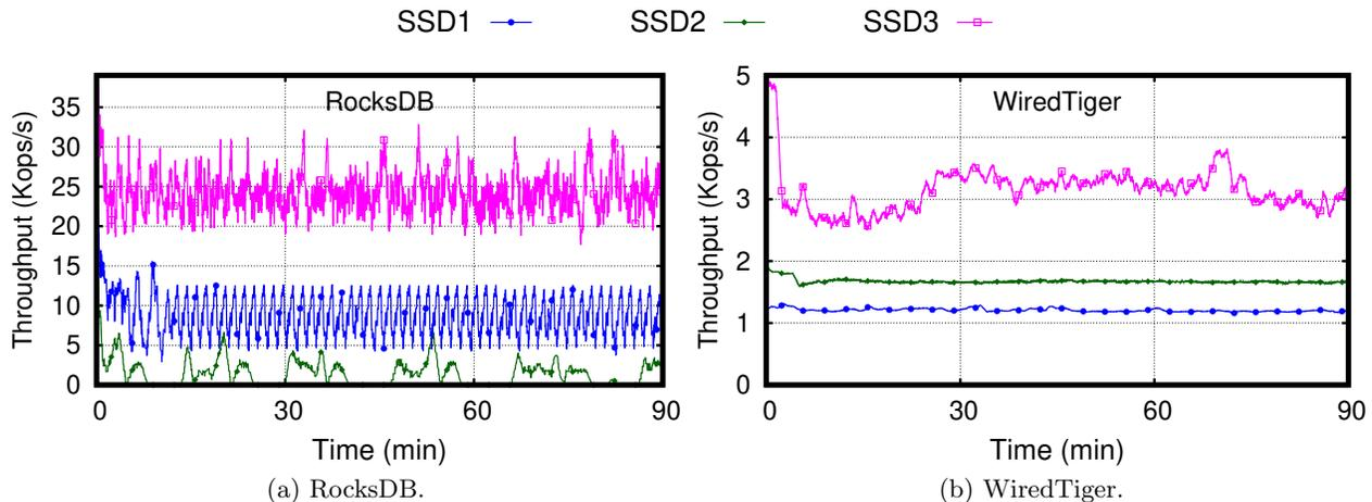
Figure 10: Throughput (1 minute average) of RocksDB (left) and WiredTiger (right) over time when running on SSDs based on different technologies. The type of SSD influences heavily the throughput variability of RocksDB, and much less that of WiredTiger.
