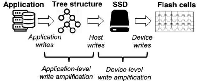
Figure 1: Write flow and amplification in PTSes. The PTS issues additional writes to the SSD to maintain its internal tree structure, which lead to application-level write-amplification. The SSD firmware performs additional writes to overcome the lack of in-place update capabilities of flash memory, which lead to device-level write amplification.
