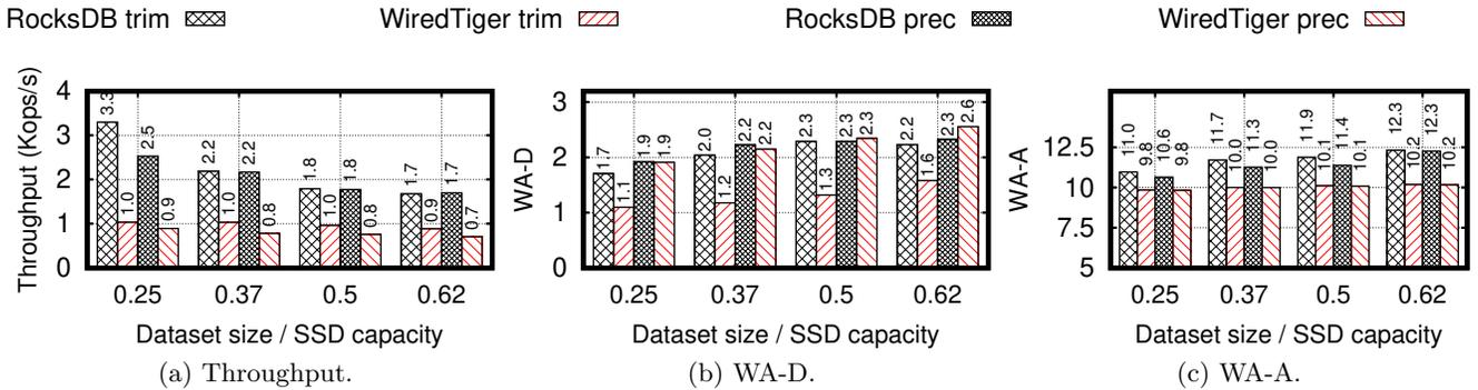
Figure 5: Impact of the size of the dataset in RocksDB and WiredTiger, with preconditioned and trimmed device. Larger datasets lead to a lower throughput (a). This is mostly due to an increase in WA-D (b), since the WA-A only increases mildly (c).
