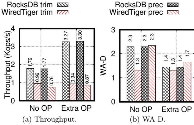
Figure 7: Impact of using extra SSD over-provisioning (OP). Extra OP may increase throughput (a) by improving WA-D (b), at the cost of reducing the amount of data that the SSD can store.
