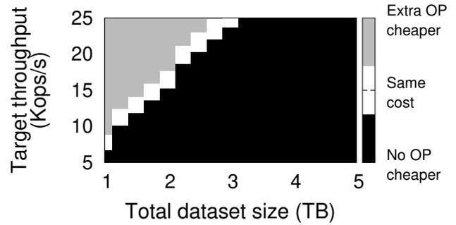
Figure 8: Storage cost comparison of using RocksDB with or without extra over-provisioning (OP) on a preconditioned SSD. The heatmap reports the RocksDB configuration that requires fewer drives to store a given dataset while achieving a target throughput –hence incurring a lower storage monetary cost.
