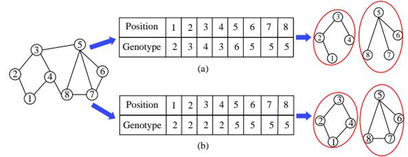
Fig. 2. An example of the locus-based encoding and label-based encodings. (a) Locus-based encoding. (b) Label-based encoding.
