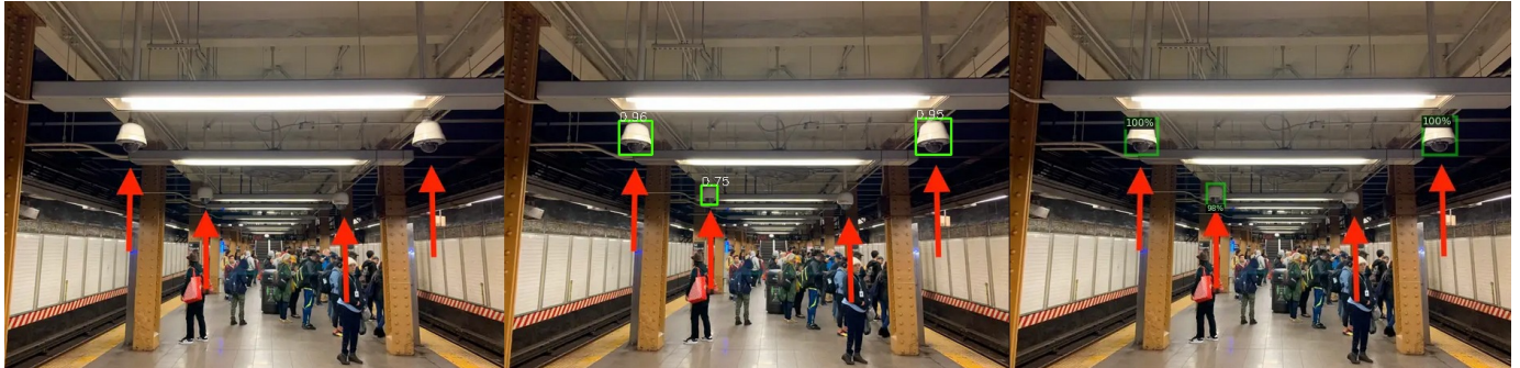
Fig. 28: Visual results (left to right): Original image (Ground Truth) - 4 TP; ATSS X-101 - 3 TP, 1 FN; TridentNet R-101 - 3 TP, 1 FN
