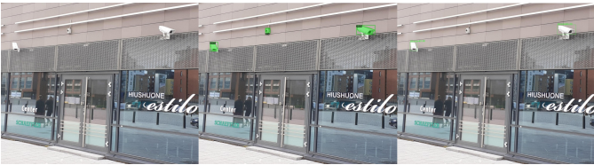
Fig. 8: Visual results (Ground Truth - 2 TP) (left to right): ResNeSt - 2 TP (2x100%), 1 FN 93%; DetectoRS - 2 TP (100% and 96%)
