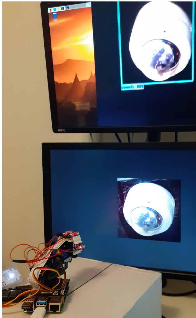
Fig. 22: Mobile device prototype in action – camera detected, lasers activated. Top screen shows the RPi4 internal view. Bottom screen shows a CCTV camera instance to test the mobile device.
