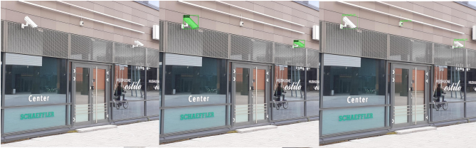
Fig. 7: Visual results (Ground Truth - 2 TP) (left to right): ResNeSt - 2 TP (2x100%); DetectoRS - 2 TP (2x100%), 1 FN 74%
