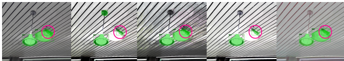
Fig. 12: Visual results (Ground Truth - 1 TP) (left to right): Original - 1 TP 88%, 2 FP (99% and 96%); Contrast - 1 TP 97%, 2 FP (99% and 96%); Equalizer - 1 TP 93%, 2 FP (99% and 80%); Exposure - 1 TP 65%, 1 FP 99%; Saturation - 1 TP 52%, 2 FP (96% and 92%)
