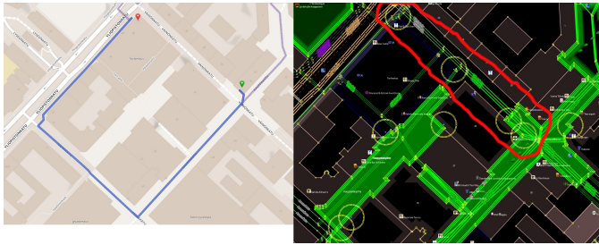
Fig. 14: Excerpt from our working prototype : CCTV-aware routing system providing route for “ Avoid CCTV Cameras (privacy-first) ” user option – CCTV-aware customization and cameras locations enabled.
