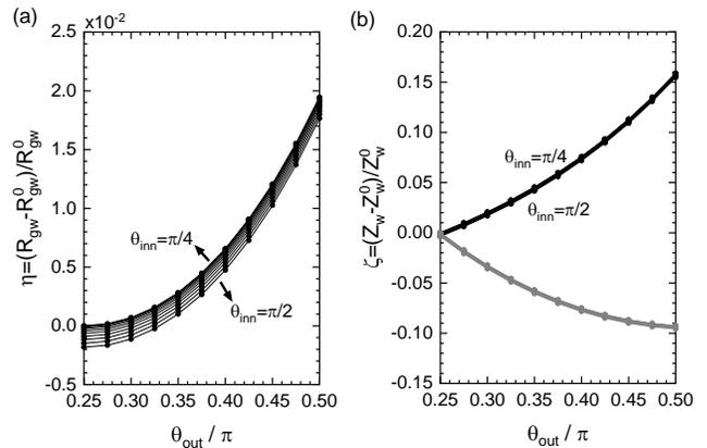
FIG. 4. Improvement ratios,  $\eta$  and  $\zeta$ , for the case of  $\ell_{out}/a_{out} = 1.2$  and  $\ell_{inn}/a_{inn} = 0.8$ . (a)  $\eta$  as a function of  $\theta_{out}$ . (b)  $\zeta$  as a function of  $\theta_{out}$ . Upper (black) and lower (gray) branches correspond to the results with respect to the axis-1 and axis-2 depicted in Fig. 1(b), respectively.
