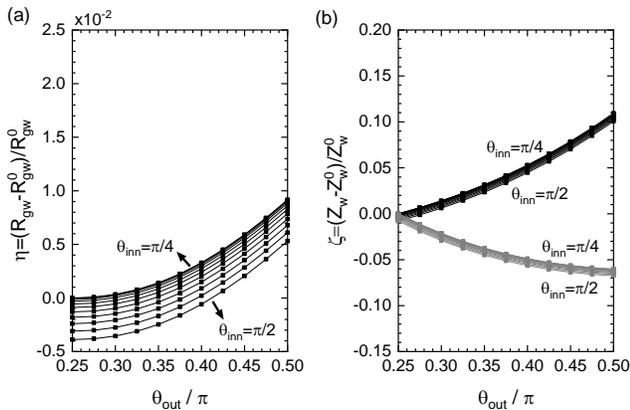
FIG. 5. Improvement ratios for the case of  $l_{\text{out}}/a_{\text{out}} = 0.8$  and  $l_{\text{inn}}/a_{\text{inn}} = 1.2$ . (a)  $\eta$ ; (b)  $\zeta$ .
