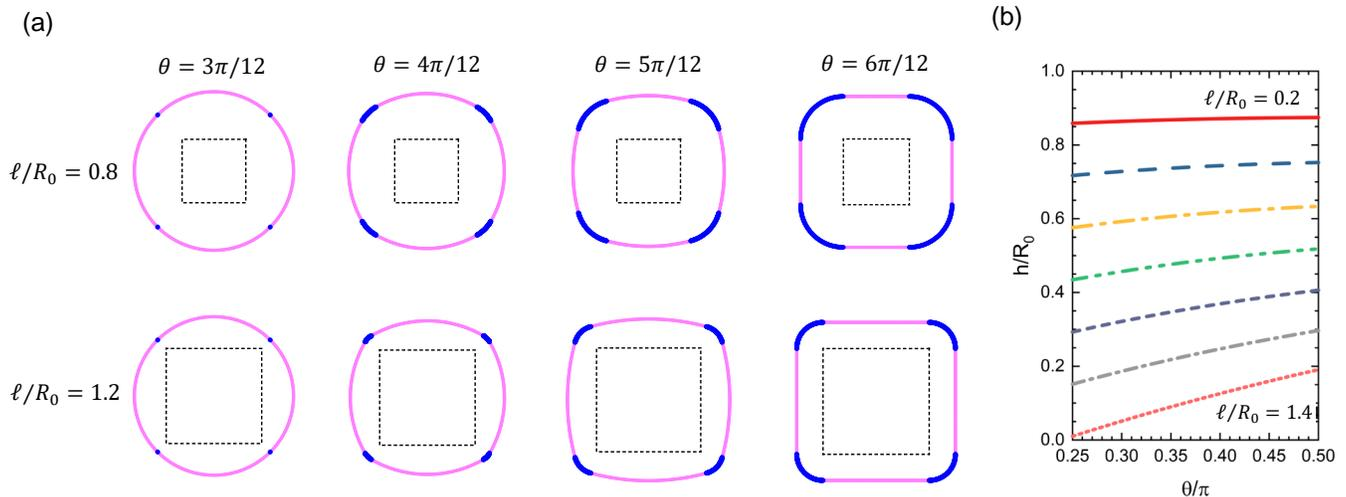
FIG. 3. (a) Geometric variation of a rounded square due to changes in variables  $\theta$  and  $\ell$  under the condition where the enclosed area  $A = \pi a_0^2$  is fixed. The constant  $a_0$  serves as the unit of length. Dotted lines show the reference squares with side length  $\ell$ . (b) Dependence of the small sector's radius  $h$  on  $\theta$ . The value of  $\ell/a_0$  is varied with interval of 0.2.
