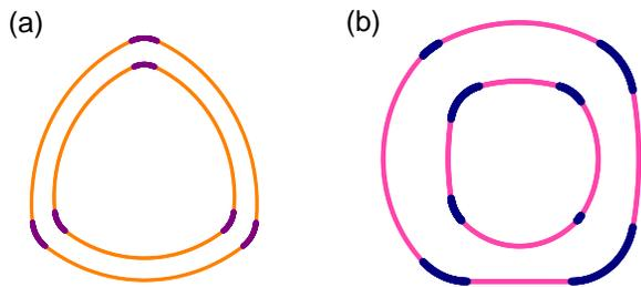
FIG. 6. (a) A model of triangular cross section with rounded sides and filleted corners, mimicking the cross section of a papyrus; see Fig. 1. (b) A model of non-symmetric hollow square cross section.
