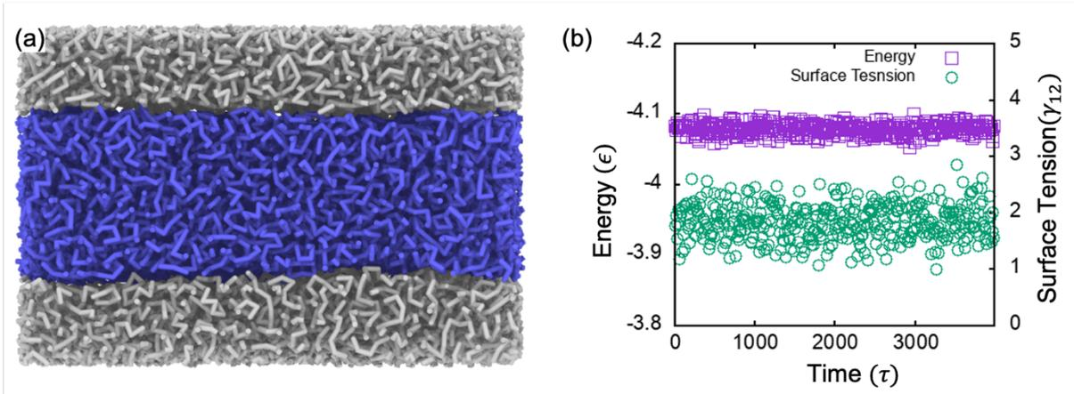
Figure 1: A polymer blend: (a) MD snapshot of two immiscible homopolymers forming interfaces in a MD simulation box. (b) energy and surface tension of the system is shown as a function of time during the production run. The energy, time and surface tension values are in LJ units.
