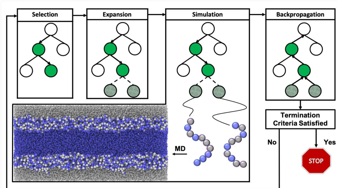
Figure 2: MD-MCTS design scheme for copolymer. It comprise of four steps – selection, expansion simulation and backpropagation that are sequentially conducted as shown by the errors in a given iteration. In the simulation step, MD calculations of a set of candidate structures are conducted parallelly. In the MD snapshot, homopolymers are shown as lines; and copolymers are shown as beads. The termination criteria is chosen to be  $\gamma_{12} \approx 0.0$ .
