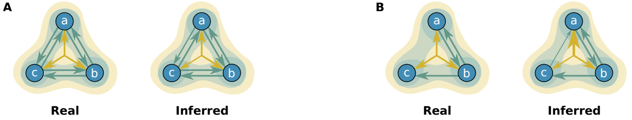
FIG. 28. Inference of directed pair and triplet couplings among three Van der Pol oscillators from the method in Ref. [424]. An arrow from the center to a node i indicates a directed triplet interaction from (j, k) to i . Panels (A) and (B) show two examples of the original structural network and the reconstructed one. While the inference in the first case is good, the method yields a spurious links from node c to a . Figures adapted from Ref. [424].
