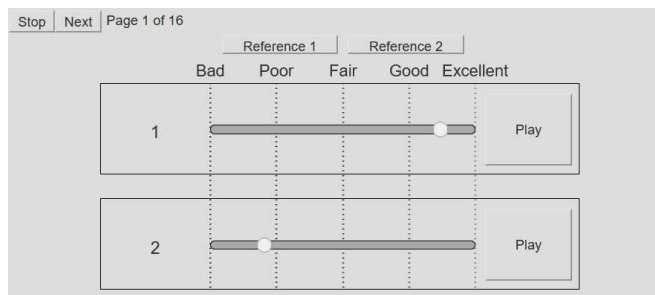
FIG. 1. Web Audio Evaluation Tool user interface used for remote testing. Shown with two file pairs.
