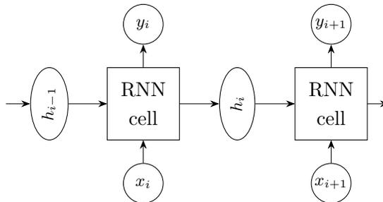
**Figure 2** Basic structure of an (unfolded) RNN.
