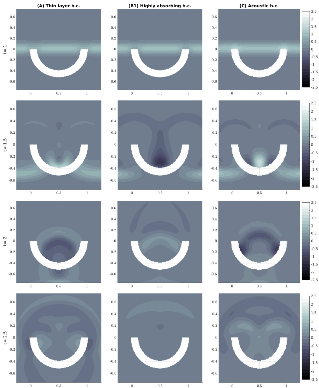
FIG. 3. Scattering of a plane wave from a "halfpipe" shape, with height 0.5, where each column represents a different boundary condition. Shown is the plane z = 0.25 , the middle of the scatterer.
