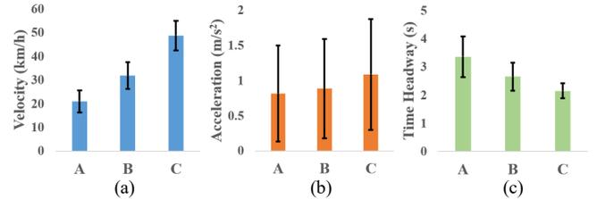
Fig. 2. Characteristic analysis of different driving styles with the NGSIM data: (a) velocity; (b) acceleration; (c) time headway. The three driving styles are denoted by, A: conservative, B: normal, and C: aggressive, respectively.
