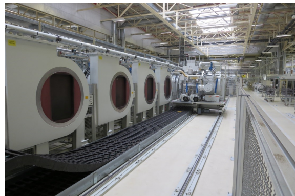
Figure 1: A steel hardening production line in Škoda Auto consisting of electrical vacuum furnaces (Dušek, 2016).
