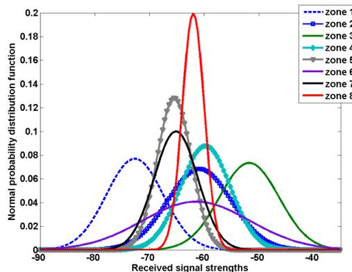
Fig. 1: Fitted distributions representing eight zones with respect to an AP.
