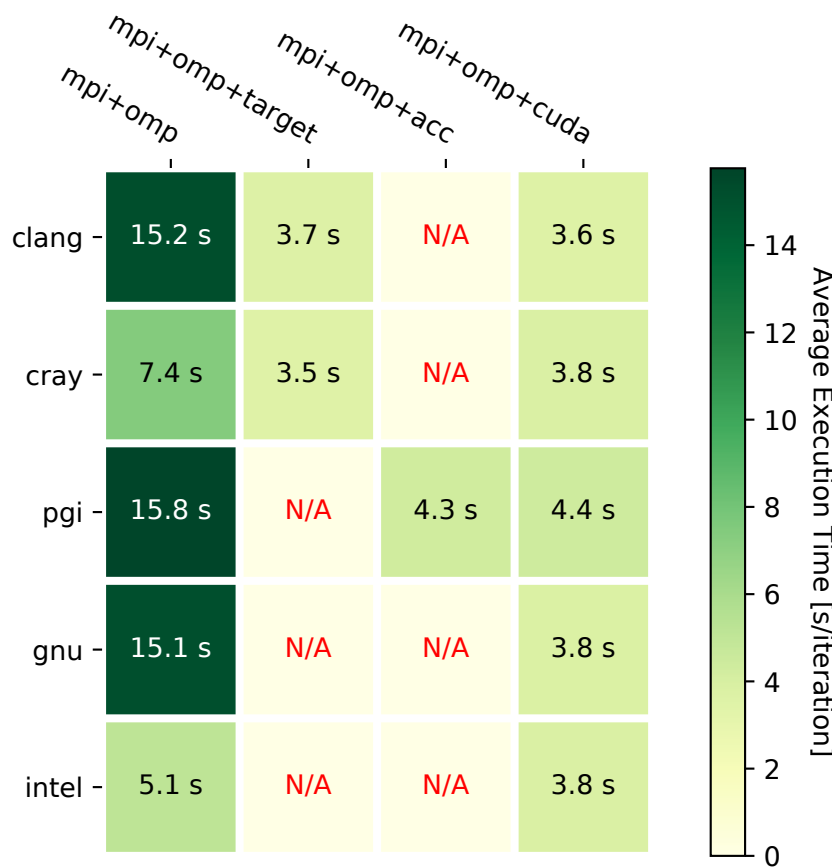
Figure 5: Average execution time per time-step for 5 compilers and for every parallel programming model available in the SPH-EXA mini-app.
