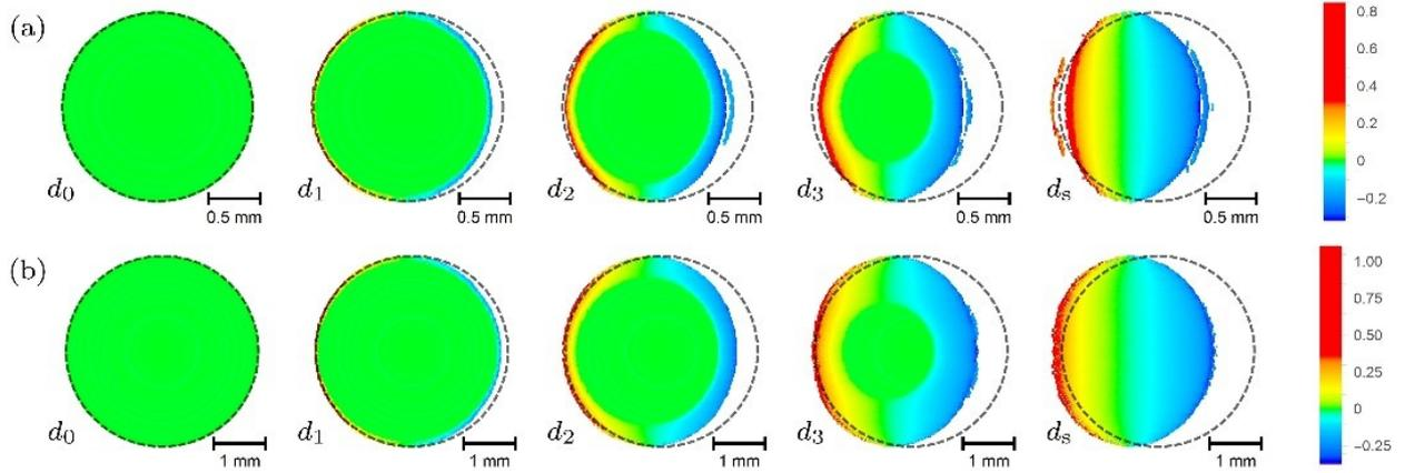
Figure 7: Evolution of the field of surface dilation/compression,  $(A^i - A_0^i)/A_0^i$ , shown in the frame attached to the moving rigid plate for (a)  $P = 0.27$  N and (b)  $P = 2.12$  N, and for the same select displacements as in Fig. 6. Dashed circles indicate the boundary of the initial contact zone. The leading edge is on the left.
