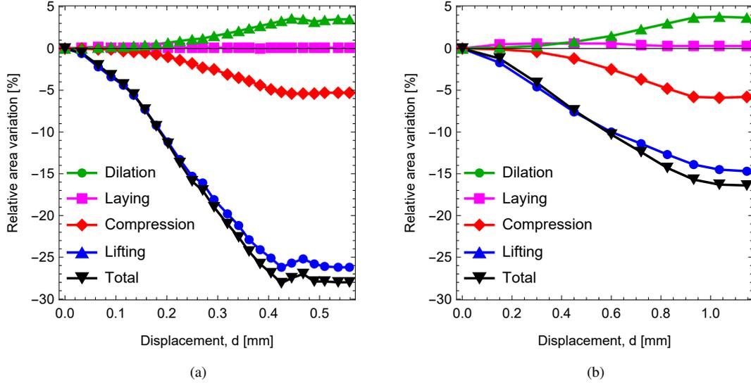
Figure 8: Evolution of the individual contributions of the various elementary mechanisms to the total relative area variation,  $\Delta A/A_0$ , as a function of the rigid plate displacement,  $d$ , for (a)  $P = 0.27$  N and (b)  $P = 2.12$  N.
