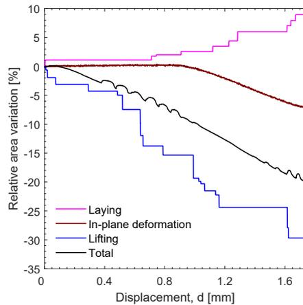
Figure 14: Contributions of the various mechanisms to the area variation. Relative area variation,  $\Delta A/A_0$ , vs the imposed displacement,  $d$ . Black: reduction of the total contact area. Blue (resp. pink): area lost (resp. gained) by lifting (resp. laying), measured as in Fig. 13. Brown: area variations due to slip-induced in-plane deformation, measured as in Fig. 15.
