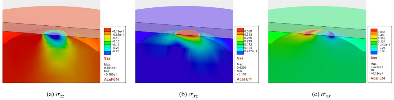
Figure A.2: Sample finite-element simulations results: components of the Cauchy stress tensor in the deformed configuration at full sliding for the neo-Hookean model.  $P = 2.12$  N. All stresses indicated in the boxes are in MPa. The leading edge is on the left.
