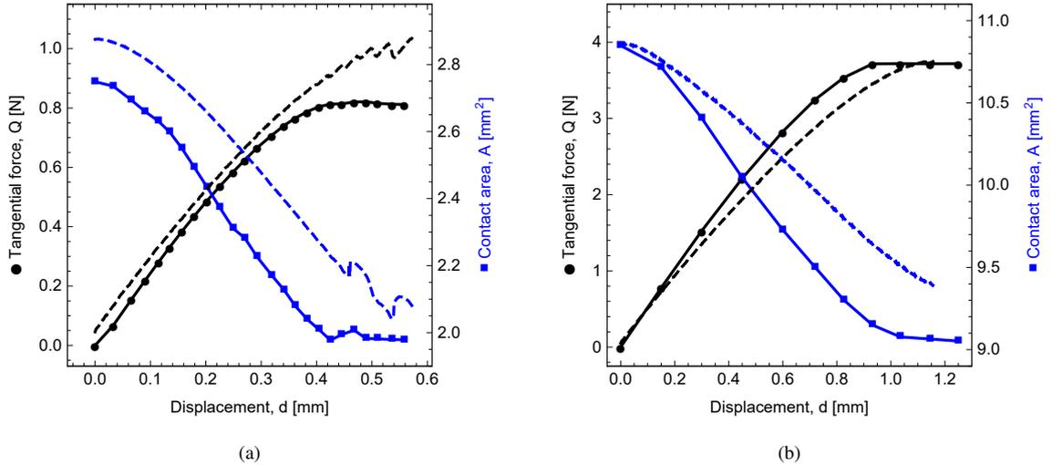
Figure S.1: Concurrent evolution of the tangential force,  $Q$  (dots), and the contact area,  $A$  (squares), as a function of the rigid plate displacement,  $d$ , for the neo-Hookean model, and for: (a)  $P = 0.27$  N, (b)  $P = 2.12$  N. Results of finite-element computations (solid lines) are compared to the experiment of Sahli et al. (2018) (dashed lines).
