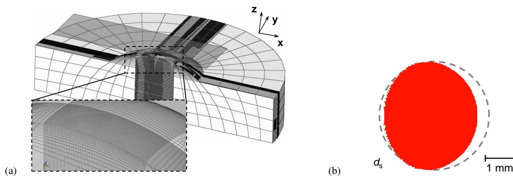
Figure S.4: Sample results obtained for the Coulomb–Orowan model. (a) Views of the mesh. (b) Contact morphology at  $d_s$  (red) compared to the initial contact (dashed circle), for  $P = 2.12\ \text{N}$ .
