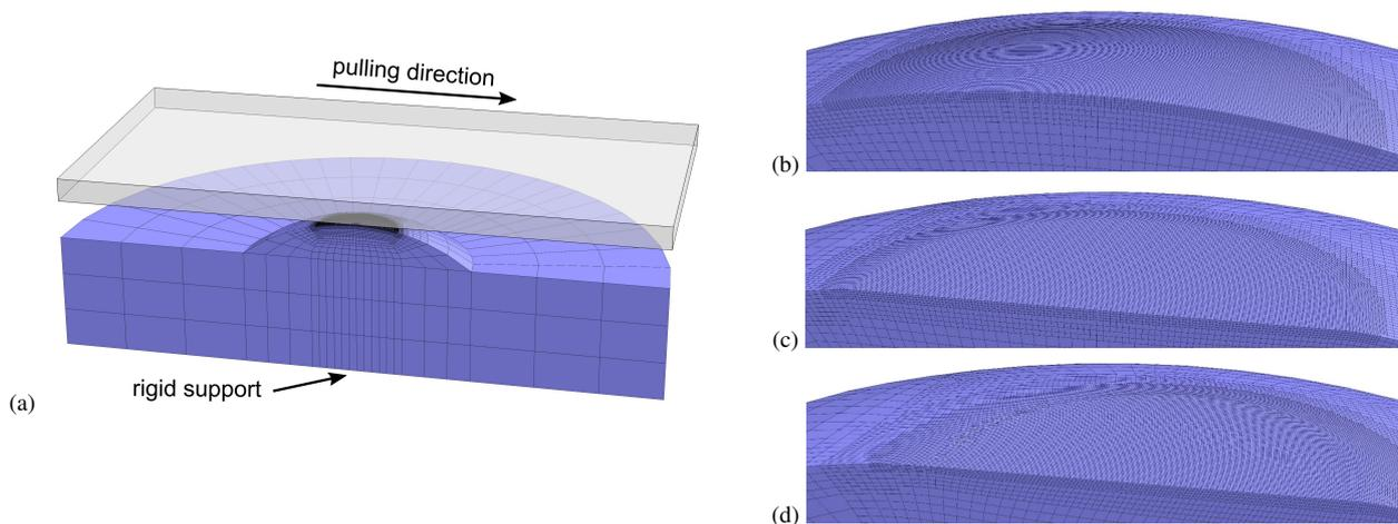
Figure 2: Finite-element mesh used in the case of the highest normal load  $P = 2.12$  N: (a) undeformed mesh, (b) zoom-in of the undeformed mesh, (c) zoom-in of the deformed mesh after initial normal loading, (d) zoom-in of the deformed mesh at full sliding. The leading edge is on the left.
