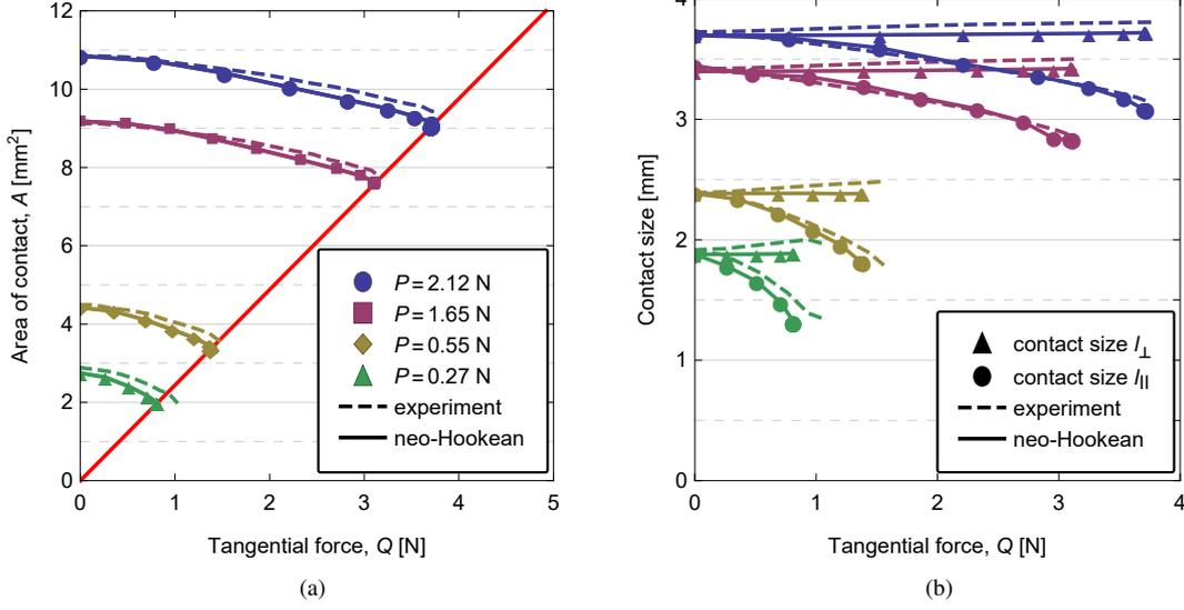
Figure 5: Comparison of the model predictions obtained for the neo-Hookean model, for all normal loads, to the experimental results of Sahli et al. (2018, 2019). (a)  $A$  vs  $Q$ . Solid straight red line:  $Q = \sigma A$ . (b) Contact size along ( $l_{\parallel}$ ) and perpendicular to ( $l_{\perp}$ ) the shear loading direction vs  $Q$ .
