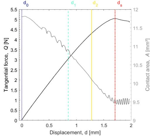
Figure 11: Concurrent evolution of the tangential force  $Q$  (solid black curve, left axis) and of the contact area  $A$  (solid grey curve, right axis) as a function of the imposed tangential displacement of the glass substrate.  $P = 1.85 \text{ N}$ .  $V = 0.1 \text{ mm/s}$ . Four values of the displacement are indicated, which will be used in further figures.
