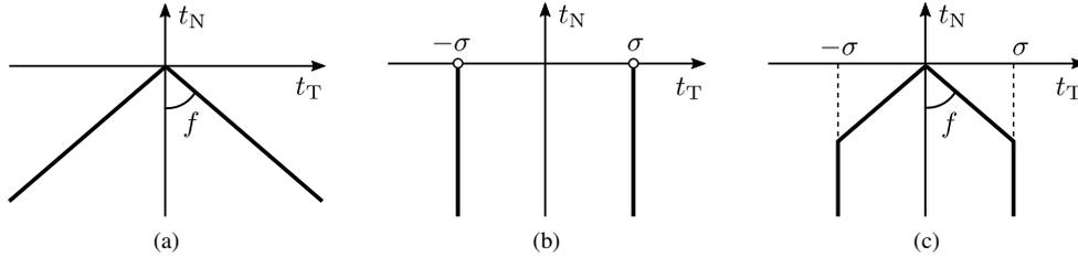
Figure A.1: Sketch of three friction laws: (a) Coulomb with a friction coefficient  $f$ , (b) Tresca with a contact shear strength  $\sigma$  and (c) Coulomb–Orowan with both a friction coefficient  $f$  and a contact shear strength  $\sigma$ .
