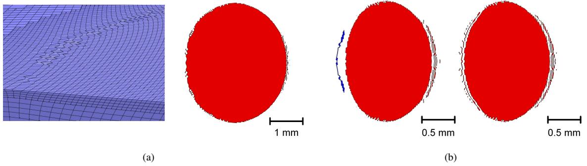
Figure S.2: Illustration of mesh-dependent features associated with the Tresca model and high contact shear strength  $\sigma$ . (a) Left: expanded view of Fig. 2(d) showing mesh distortion at the leading edge at  $P = 2.12$  N ; right: corresponding contact area with a wiggled periphery. (b) Contact area at two instants during gross sliding at  $P = 0.27$  N showing small contact spots developing and evolving outside the main contact area.
