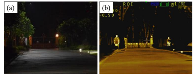
Fig. 2 (Color online). Input partial images: (a) u - image from the visible channel and (b) v - image from the IR channel
