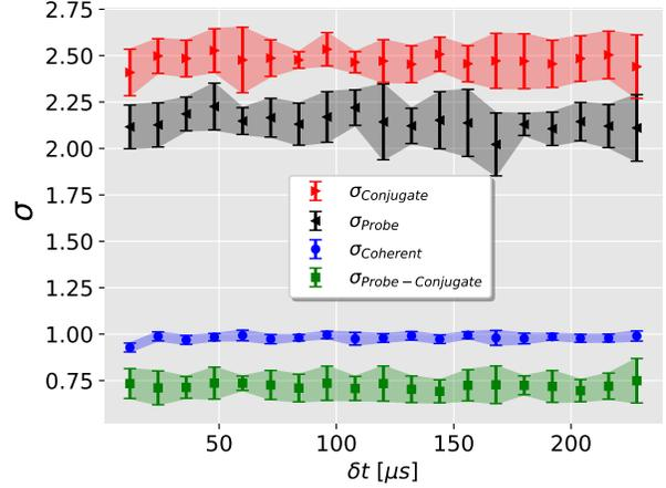
FIG. 4. The temporal quantum noise reduction characterization  $\sigma$  as a function of the time interval  $\delta t$  between successive images for different beams of light. Green squares: twin beams; blue dots: coherent beams; black triangles: probe beam only; red triangles: conjugate beam only.
