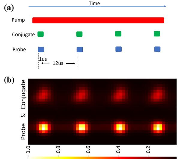
FIG. 2. (a) Time sequencing of the pump and twin beams. The pulse duration of  $1 \mu\text{s}$  and the duty cycle of  $1/12$  is realized by pulsing the probe beam with an AOM. The CW pump beam is present all the time. (b) Typical images of the twin beams captured by the EMCCD camera with four consecutive pulses.
