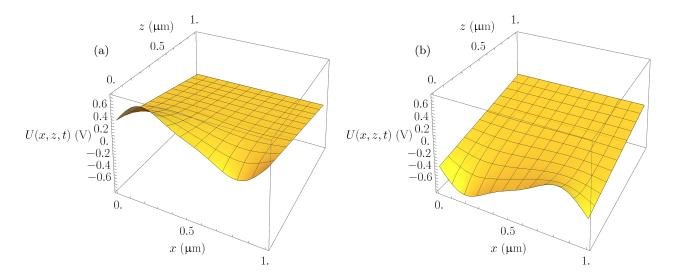
FIG. 2. The electrostatic potential landscape U flips between two landscapes: (a) one at times  $0 \le t < \tau/2$  and (b) the other at times  $\tau/2 \le t < \tau$ .
