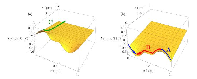
FIG. 7. Two-dimensional landscapes associated with the electrostatic potential  $U_2$  at times (a)  $0 < t \le \tau/2$  and (b)  $t > \tau/2$ . The arrows correspond to pathways that regulate the current reversal. Timescales for one-dimensional diffusion along pathways A, B, and C are reported in Table I.
