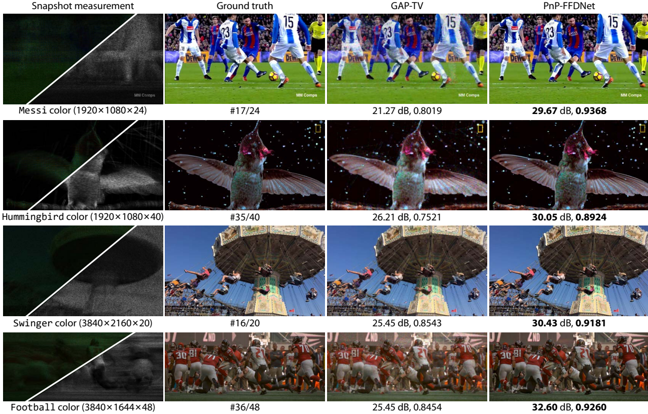
Figure 8. Reconstructed frames of PnP-GAP algorithms (GAP-TV and PnP-FFDNet) on four simulated large-scale video SCI datasets.
