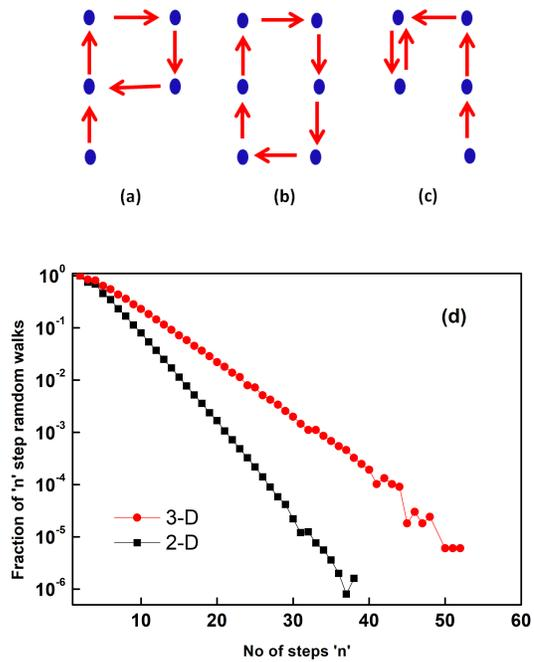
FIG. 4. (a),(b), and(c) A few examples of random walk in the 2-D model which ends up in an absorbing state. If the evolution of site A is affected by site B, we draw an arrow from site A to site B. (d) shows the fraction of walks surviving till step  $n$  in 2-D and 3-D.
