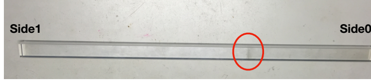
Fig. 2: BGO crystal with dimension of 25 \times 25 \times 600 mm.
