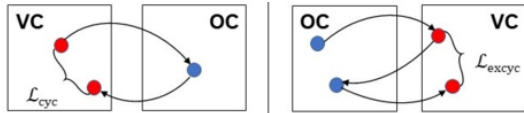
Figure 3. The image on the left depicts the cycle consistency loss used for VC to OC translation from Zhu et al’s CycleGAN [27]. The image on the right shows the extended cycle consistency loss that we used for OC to VC translation.
