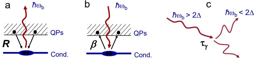
FIG. 1: Different processes governing the relaxation dynamics of photo-excited QPs in a superconductor: (a) recombination of two QPs into the condensate via emission of  $2\Delta$  boson (phonon), (b) pair-breaking by absorption of a boson, (c) decay of high energy bosons. The latter can proceed via decay of bosons into the (dielectric) substrate or via anharmonic decay into low-energy bosons, with energy less than  $2\Delta$ .
