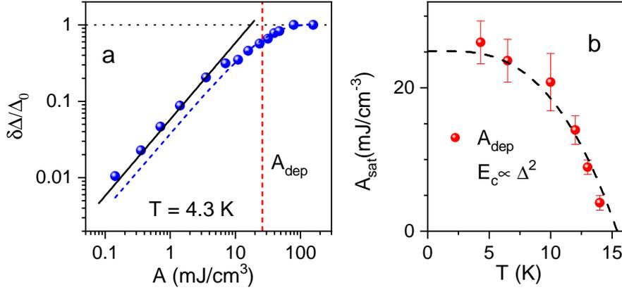
FIG. 6: (a) The dependence of the peak gap suppression,  $\delta\Delta/\Delta_0$ , in NbN on  $A$  at 4.3 K (see the traces in Figure 4a). The dashed line is a fit to the simple saturation model, the solid line is the linear fit. (b) The T-dependence of the energy density required to deplete superconductivity,  $A_{\text{dep}}$ , compared to the T-dependence of  $\Delta^2$  (dashed black line).
