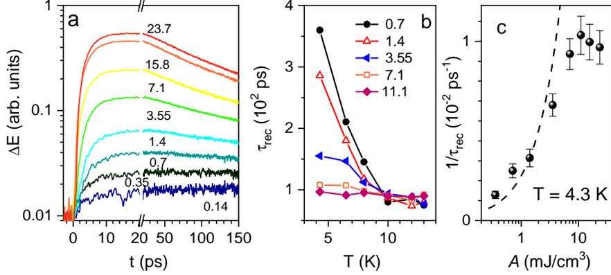
FIG. 7: (a) The time evolution of the photoinduced gap suppression (spectrally integrated response - see text) recorded on NbN thin film at 4.3 K with excitation density covering over two orders of magnitude. (b) Temperature and excitation dependence of the superconducting state recovery time,  $\tau_{rec}$ , obtained by a fit of the data in panel (a) with an exponential decay function. (c) The low temperature superconducting state recovery rate in NbN as a function of excitation density.
