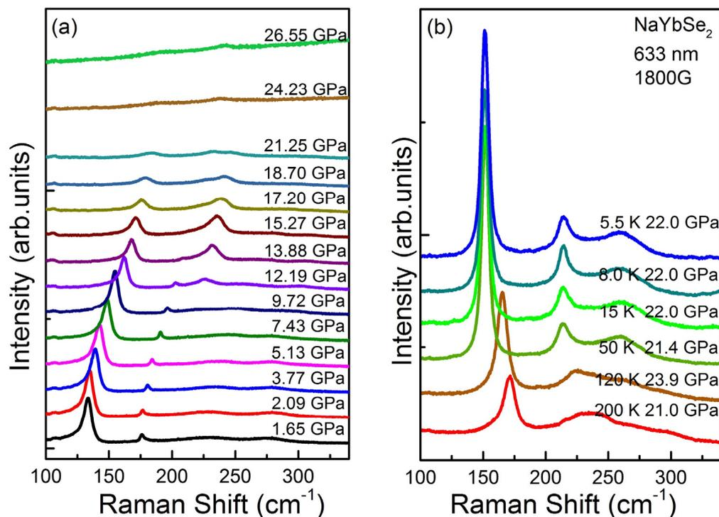
**Fig. 2** (a) High-pressure Raman spectra for NaYbSe<sub>2</sub> crystals. (b) Temperature-dependent Raman spectra with the pressure fixed at  $\sim 21$  GPa.
