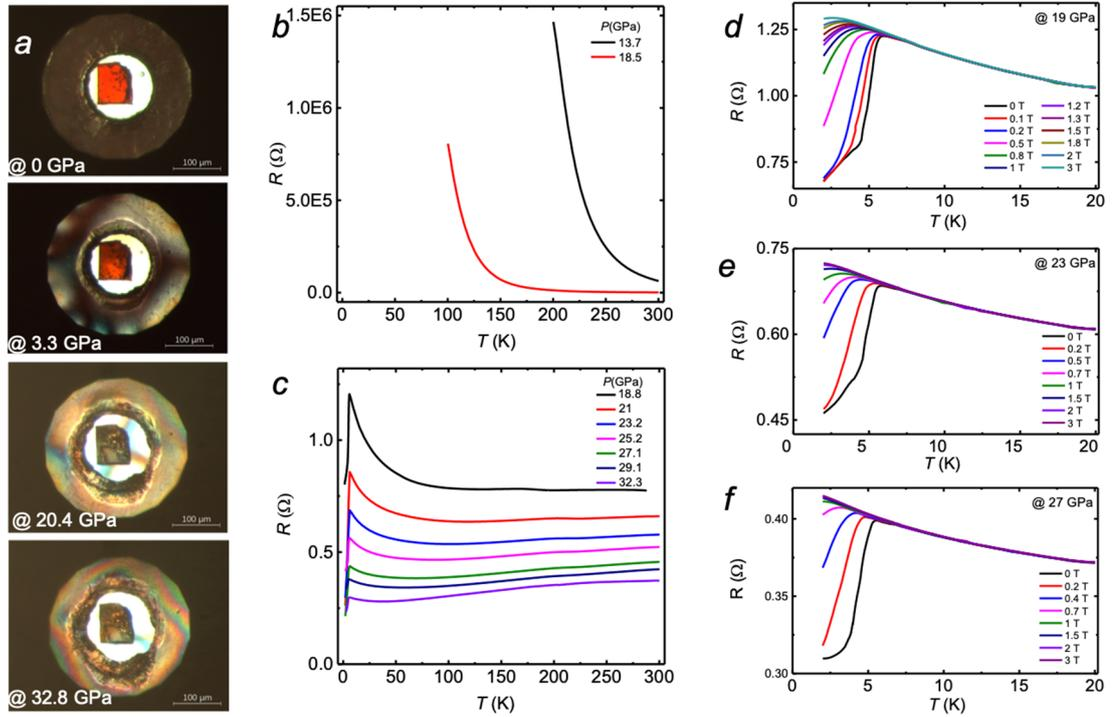
**Fig. 3** (a) Color evolution of NaYbSe<sub>2</sub> crystals under various pressures. (b) & (c) Temperature-dependent resistance under pressure. (d), (e) & (f) Evolution of SC transition under magnetic fields with the pressure fixed at 19, 23 and 27 GPa, respectively.
